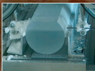
Above: cutting Antarctic ice core (bandsaw) Left: ice drilling in Antarctica (both images courtesy Eric Wolff)
