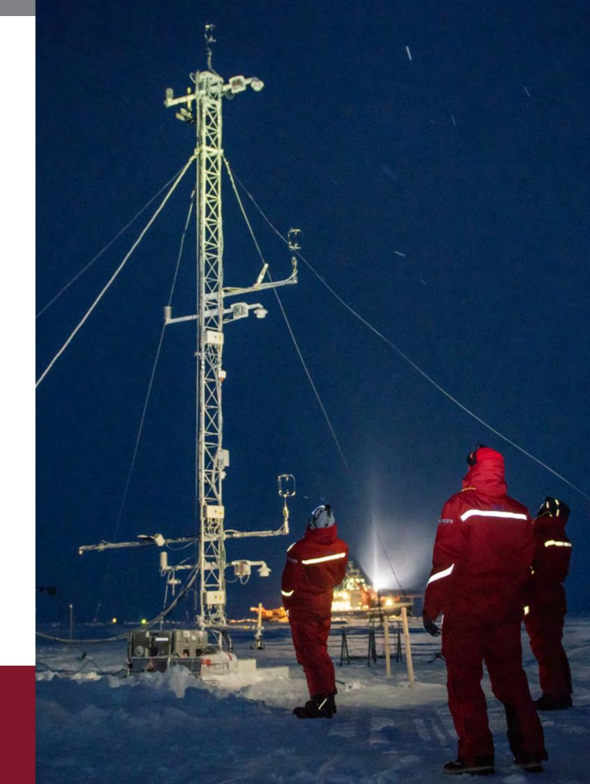
After lots of planning and preparation, the 11 meter high metrological tower at Met City was raised. From the tower, MOSAiC researchers will get a collect a range of atmospheric and surface measurements and samples.
