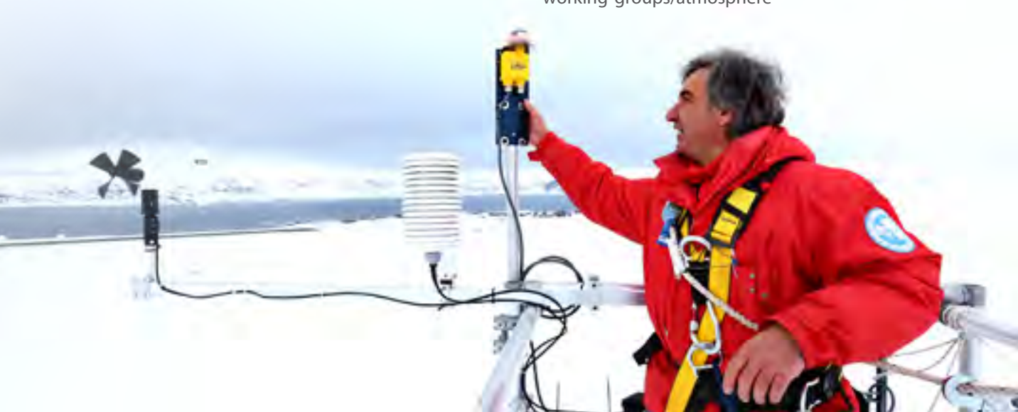
PHOTO: LUCA BRACALI Measuring chemical-physical parameters in the low troposphere on top of the Amundsen-Nobile Climate Change Tower on Svalbard. Built in 2009 by a team from the Italian National research Council (CNR), the tower has 18 floors and is 34 meters high.
