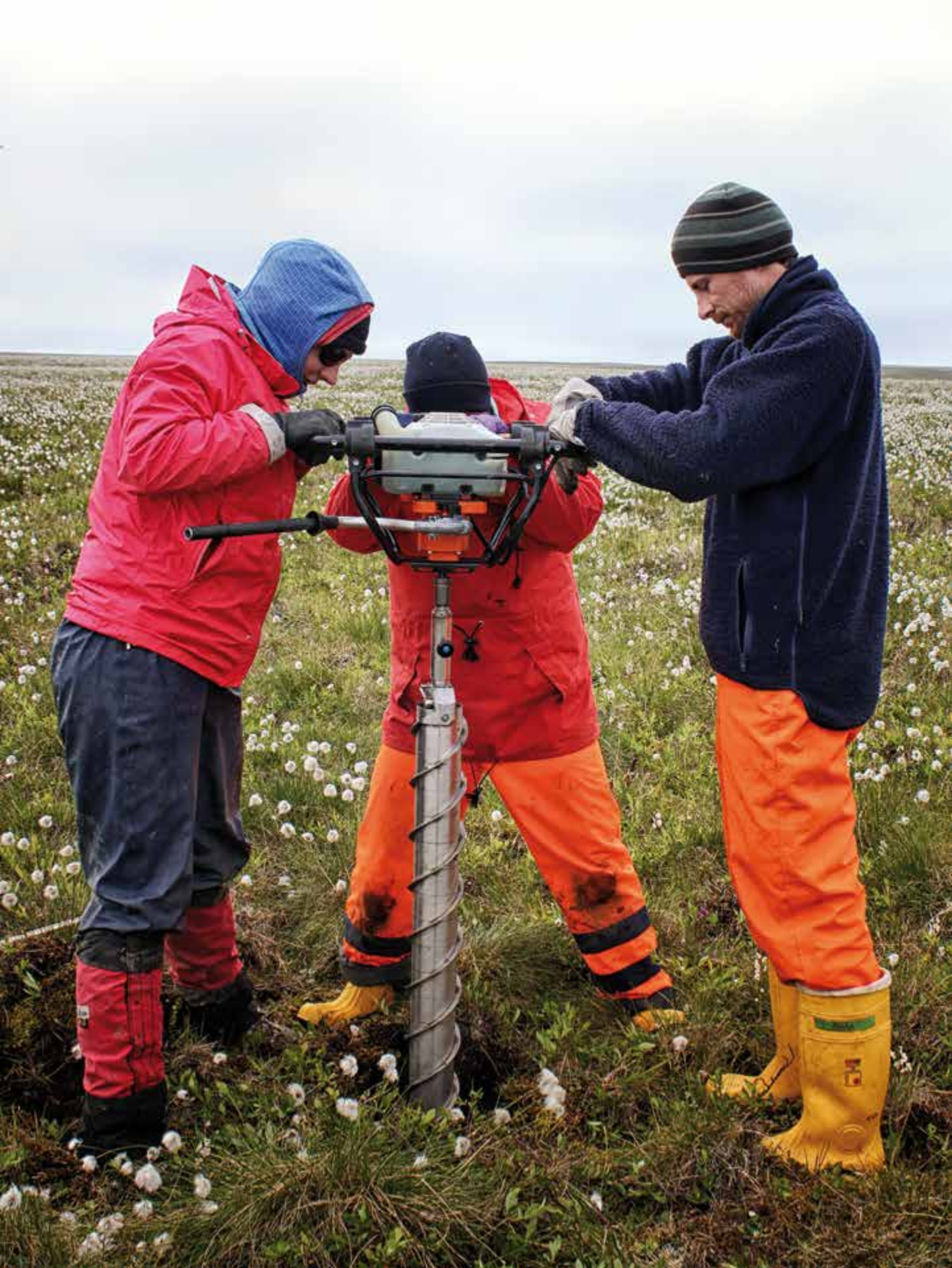
PHOTO: LOUISE BEVERIDGE Drilling of permafrost cores in Arctic tundra on Herschel Island, Canada.
