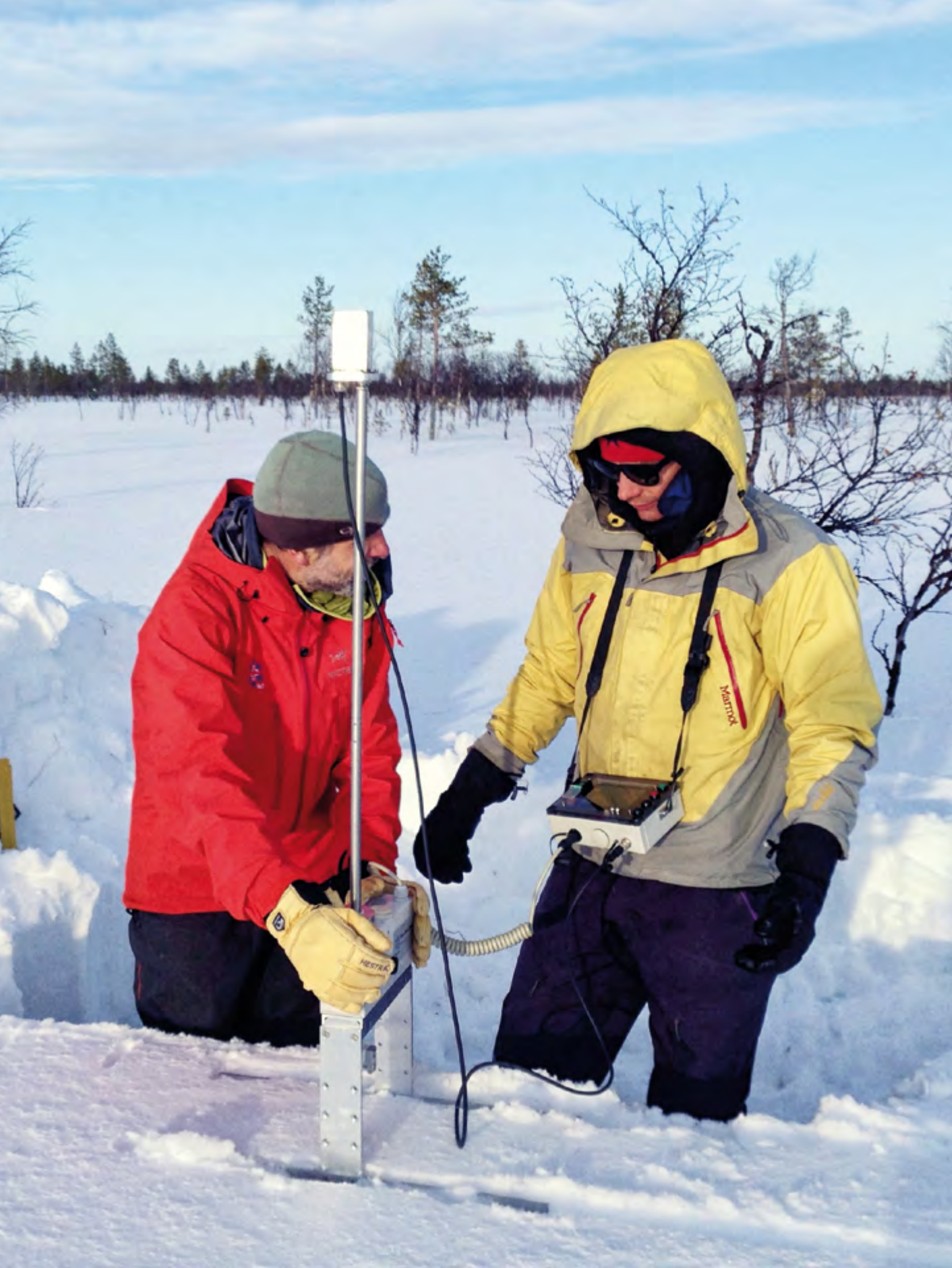
PHOTO: SVETA STUEFER Snow science winter school: Martin Schneebeli and Martin Proksch demonstrating the SnowMicroPen on the bog site of the Finnish Meteorological Institute in Sodankylä, Finland.
